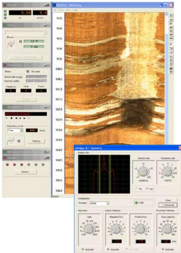
The heart of the graphical user interface is the Dashboard which consists of multiple threads running concurrently and handling specific system tasks simultaneously. The dashboard is the operator's control panel to select and control all system functions and to monitor the data acquisition process and tool status.
